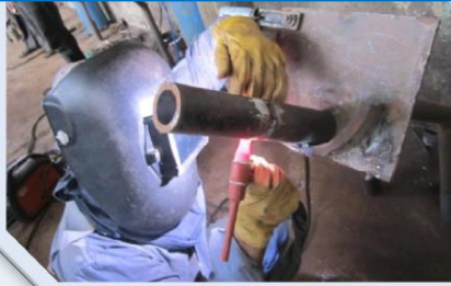
2" x SCH 160 ASTM A106 Gr B. Pipe for qualification (GTAW + SMAW)
