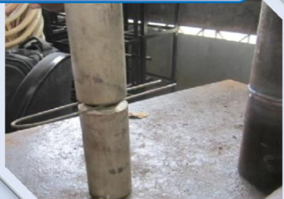
2" x SCH 160 – SS316L Pipe on setup
