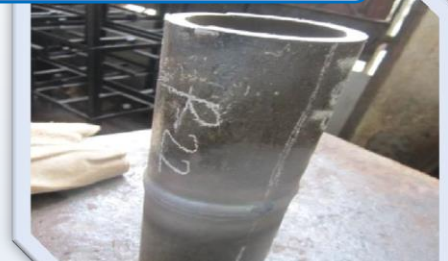
3" x SCH 80 - P22 Material (GTAW + SMAW)
